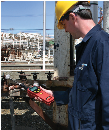
Workers can easily and quickly obtain VOC readings anywhere in the facility with the RAE Systems UltraRAE 3000+
