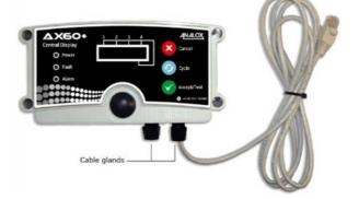
The empty gland on the left is for the power supply unit cable. A third gland must be fitted if the optional beacon is to be installed. Both of these cables must be fitted by the installer.
