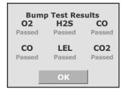
If all the sensors have passed the bump test, the instrument goes to the gasmonitoring display screen. If any sensor failed the bump test, after viewing and acknowledging the results, the instrument asks the user to continue, or calibrate the failed sensor(s). If the user selects the Cancel button, the sensor is not calibrated and the instrument moves on to the next sensor in the list. If the user selects "OK", the failed sensor is calibrated.
