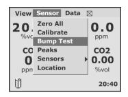
The screen to alert the user to apply gas to the instrument is then shown. The user has a fixed number of seconds to apply gas and select "Start" before the bump times out. If the user selects "Skip", the bump for this particular sensor is not done. The instrument moves on to the next sensor.
