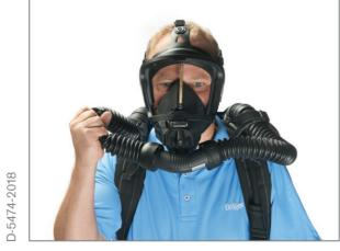
**RP with PSS BG 4 plus:** With RP mask, press the right hose together and inhale. If the negative pressure does not persist, tighten the straps. Exhaled air must escape through the left hose into the system. Only use the mask if you are sure it is sealed!
