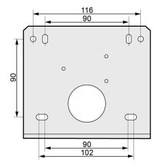
Figure 3: drilling diagram for wall mounting (view of the side flatten onto the ceiling).
