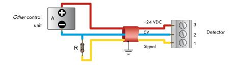
Figure 7: Connection of a 3-wire CTX300 sensor to a non-TELEDYNE OLDHAM SIMTRONICS control unit.
